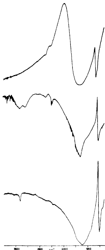
Figure 3. Infrared spectra for h-BN. (Top) highly ordered BN. (Middle) polyborazinyamine pyrolysis product formed in a nitrogen atmosphere at 900 °C and briefly fired at 1200 °C in air. The weak band at \sim 3200\text{ cm}^{-1} corresponds to a BOH band due to partial oxidation. (Bottom) polyborazinyamine pyrolysis product formed in an ammonia atmosphere at 1200 °C. The peak at \sim 3480\text{ cm}^{-1} indicates residual N-H groups.
